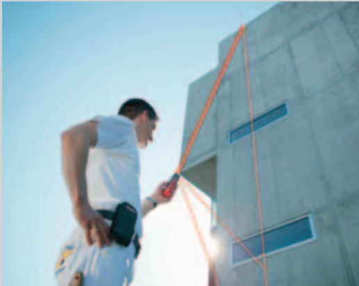
Indirect height-measurement: determine facade heights using the Pythagoras function
